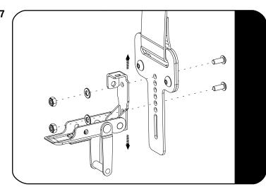
Using an 3mm allen key and a 7mm spanner, loosen the two bolts holding the latch to the latch plate.
