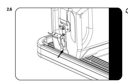
Open the latch and hook it into the catch plate on the Jerry Can Holder Tray.
