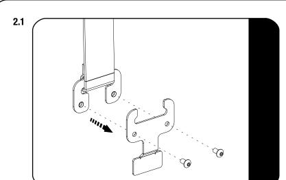
Remove the rear hold plate on the stap.
