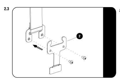
Assemble the Long Rear Holder Plate to the strap as shown.
