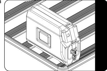
Engage the latch to secure the Water Jerry Can in place.
